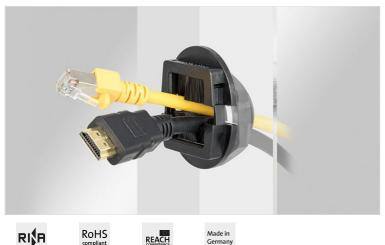
For round metric cut-outs M32/M50 icotek offers the split cable gland with brush strips KEL-BES-S round. It can be either directly snapped into the cut-out or screwed with a locknut, which is included in the shipment.
